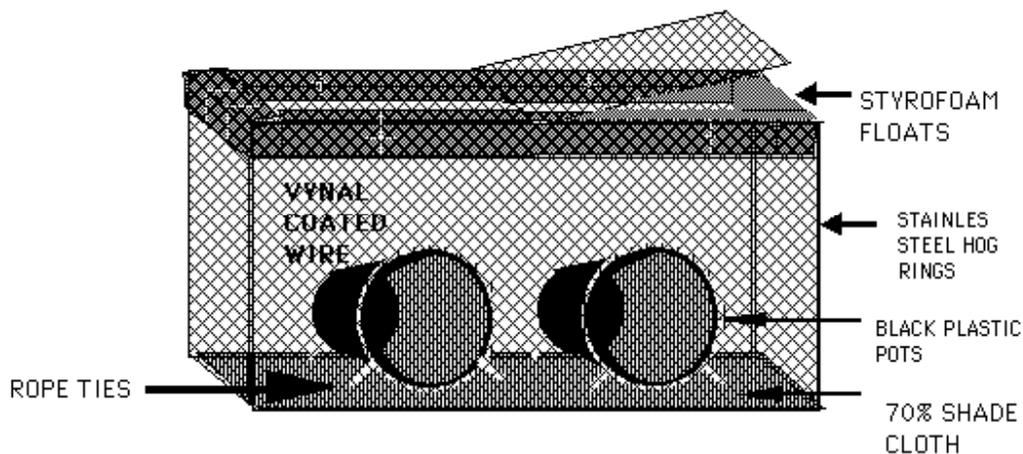
**Figure 20. Breeder Cage with Description of Materials**
