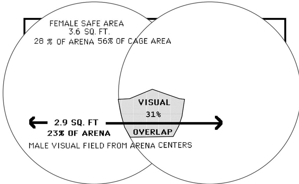
IN THIS SECOND EXAMPLE THE SAFE AREA OF THE TOTAL CAGE FOR THE FEMALES IS SHOWN TO BE 56% AGAINST 62.5% OF THE FIRST CAGE. IF HOWEVER THE SAFE AREAS IN CAGE ONE ARE COMPARED AGAINST THE UNSAFE AREAS IN THE SAME CAGE AS A RATIO, WE FIND THAT THE RATIO OF SAFE TO UNSAFE AREAS IS 1.92 AS COMPARED WITH A RATIO OF 1.25 IN THIS EXAMPLE.
