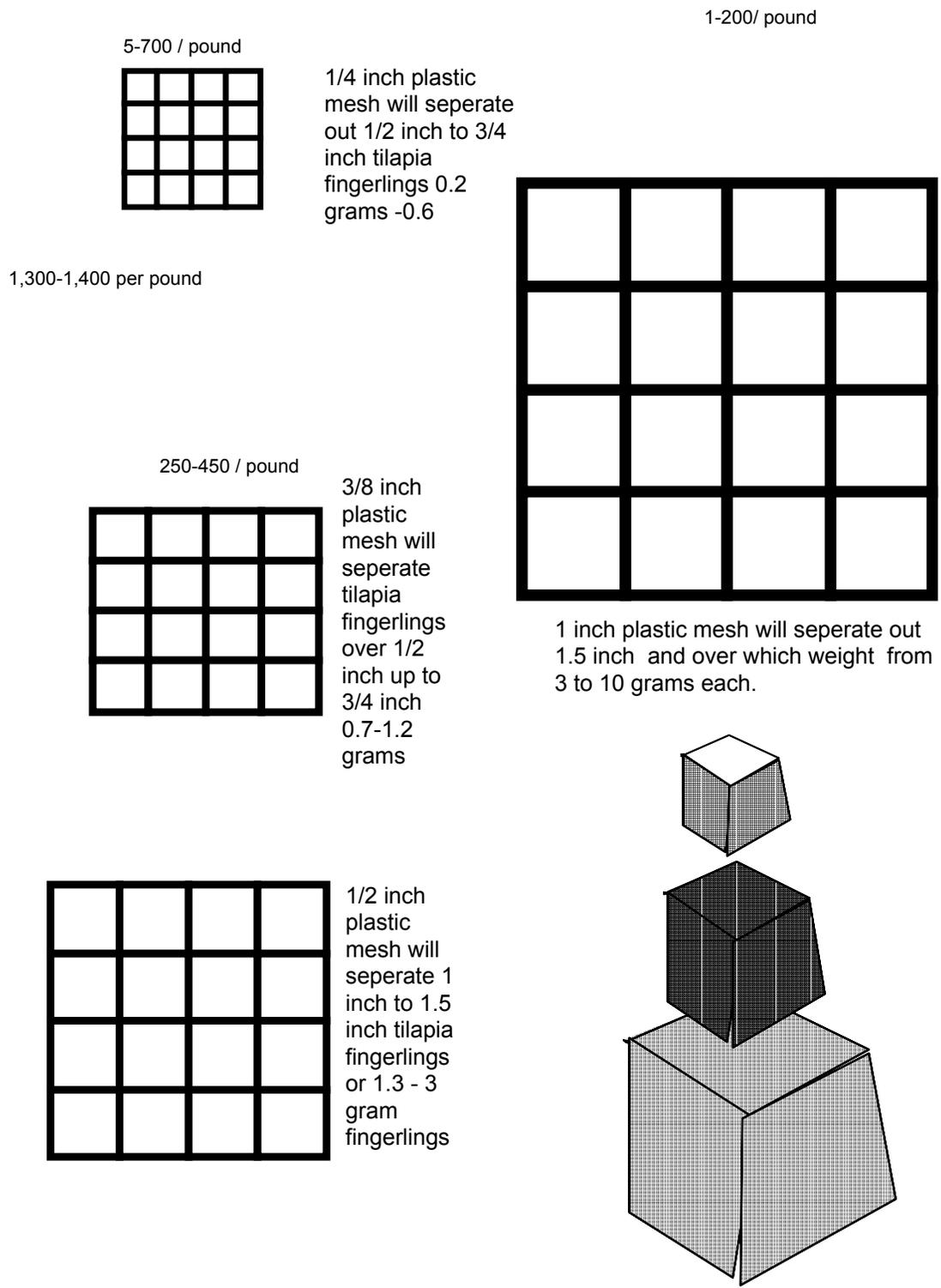
**Figure 16. Mesh for Grading Fingerlings**
