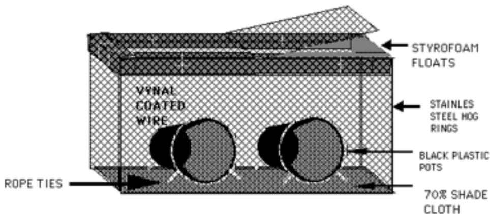
The cage material can also be plastic and can be square mesh one inch and solid enough to take the handling the cage will have.
